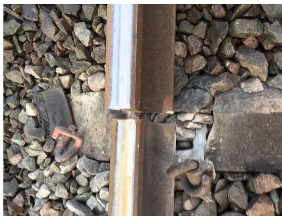
Figure 1 Typical photo of a broken rail demonstrating the 'clean' nature of the break
