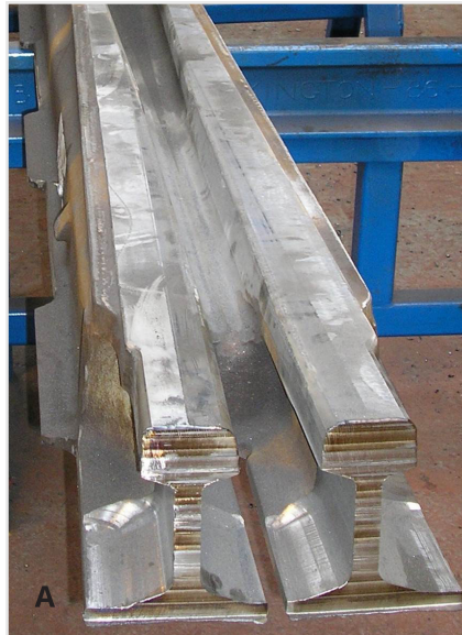
Image 6: Traditional (a) and continuous flange (b) designs
