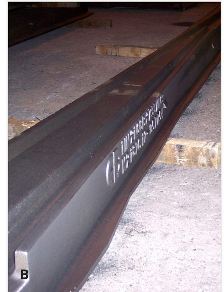
Image 6: Traditional (a) and continuous flange (b) designs
