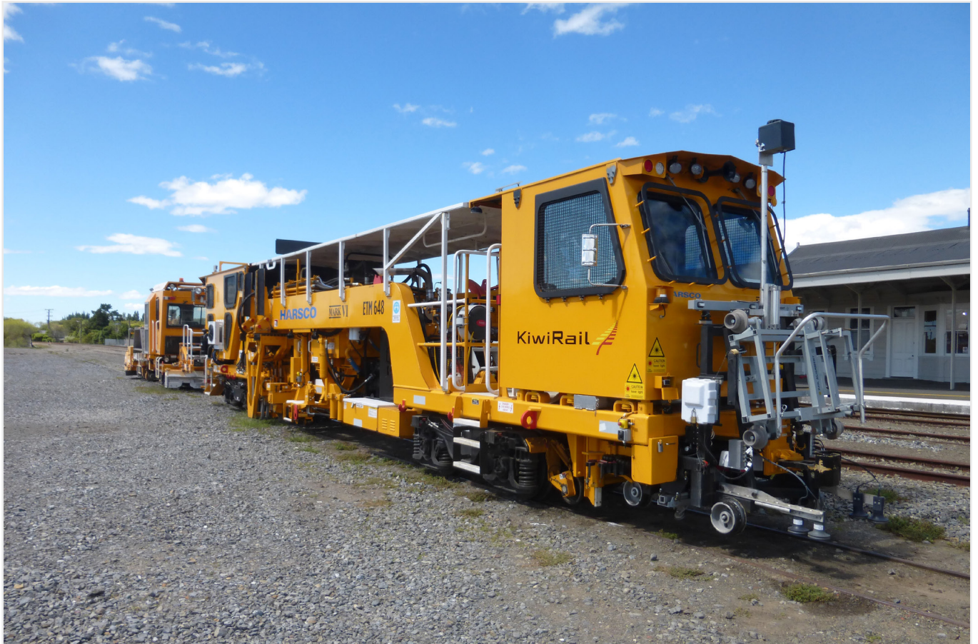
Image 9: KiwiRail Harsco MkVI tamping machine and ballast Regulator. Photo by Phil Kirkland
