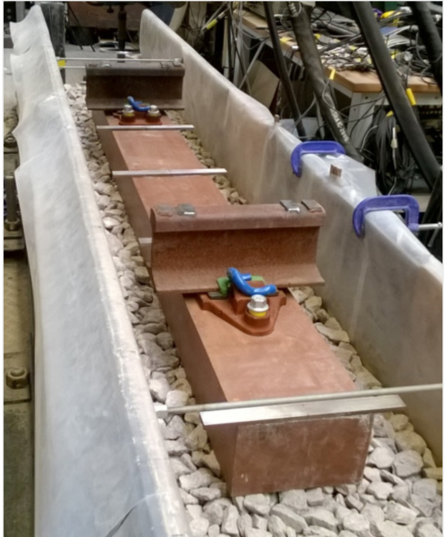
Figure 3. Photo of the composite sleeper tested (steel plates were attached to allow the installation of the LVDTs)
