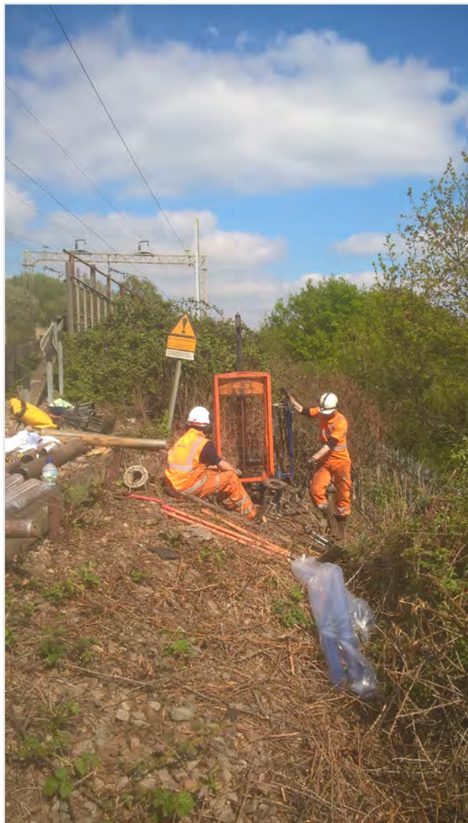
A) LLAMAR Rig set up at embankment crest at Country end of site for window sampling
