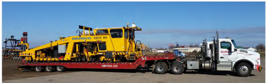
Newly delivered Harsco Mark 1V HD tamping machine. Image: Arctic Gateway Inc.
