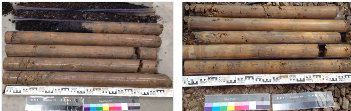
Figure 9: Embankment fill material encountered during 2015 GI works
