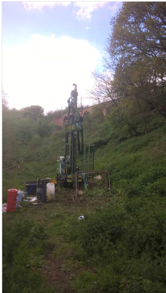
B) Rotary rig set up at embankment toe at London end of site for continuous sampling
