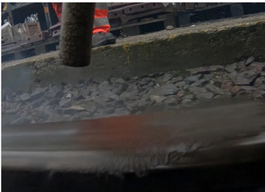
Image 4: A still from the nozzle camera showing water being removed from the railhead.
