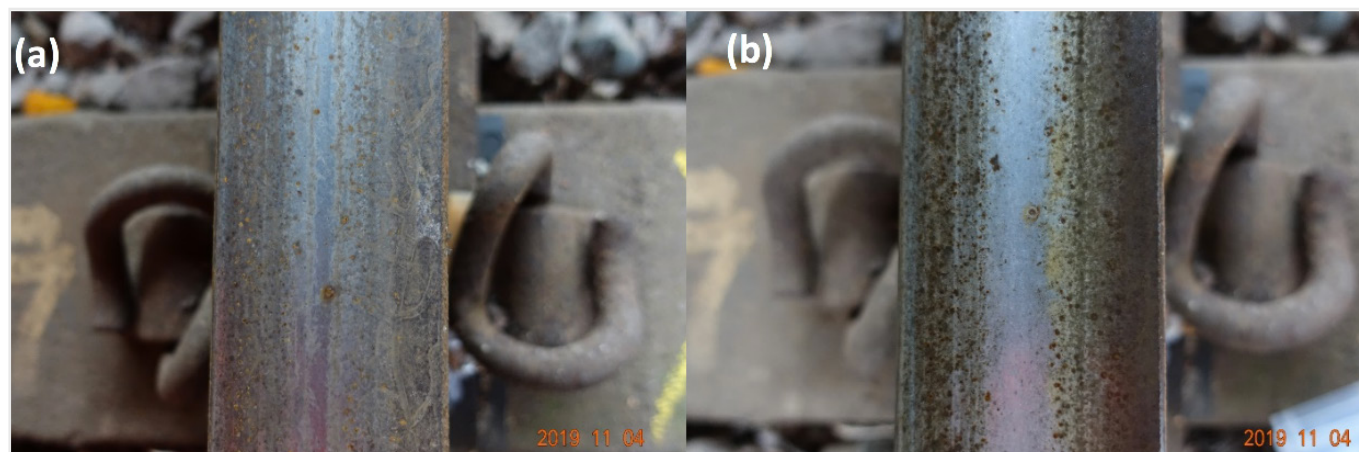
Image 7: Contaminated untreated railhead (a), treated cleaned railhead (b)
