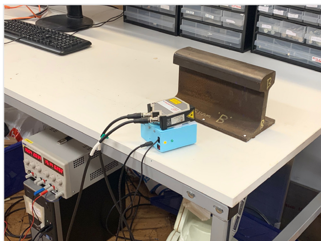
Figure 7: Handheld rail profile scanner.
