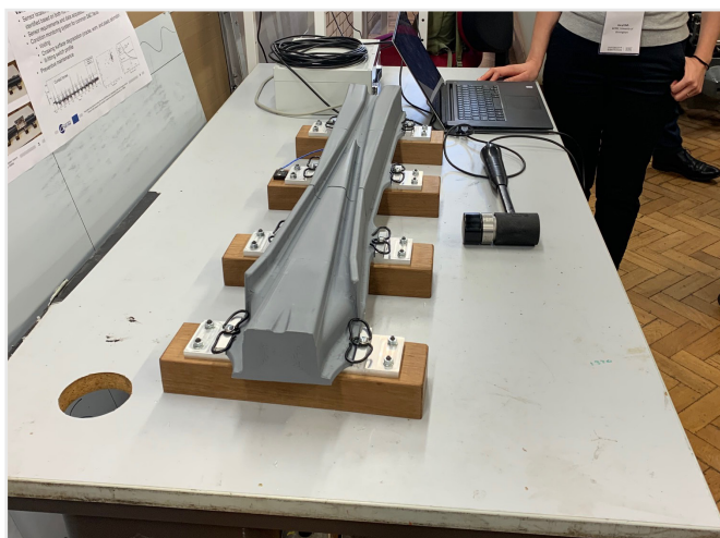
Figure 6: Demonstration of embedded sensors within crossing nose.
