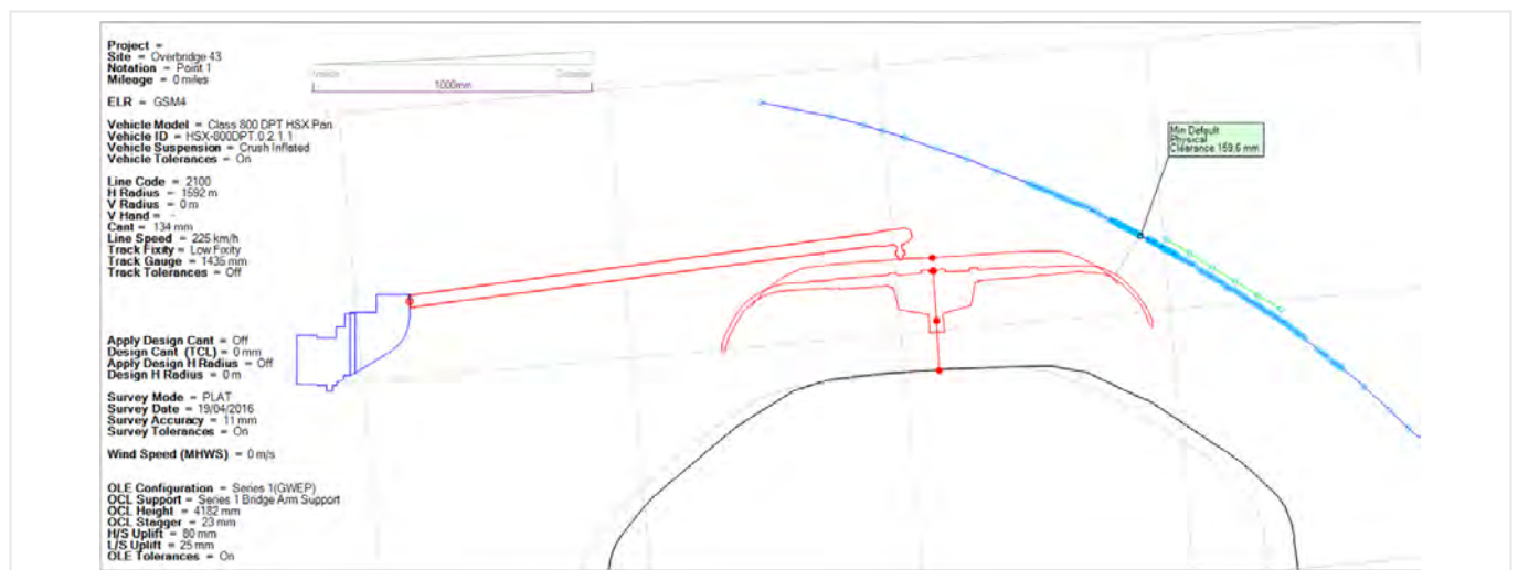
Figure 4: Clearing Actual Pantographs - An example of the electrical clearance at Old Dalby and actual rolling stock.
