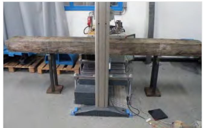
Figure 10: Three-point bending testing of 150(h) x 250(w) mm oak sleeper (span 1435 mm, loading speed 76 mm/min).
