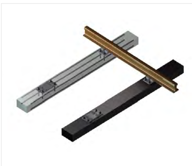
Figure 4: Steel bar reinforced polymer sleeper, showing 4 reinforcement bars.
