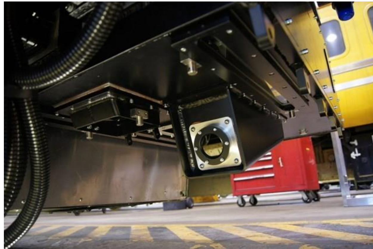
Plain Line Pattern Recognition camera
