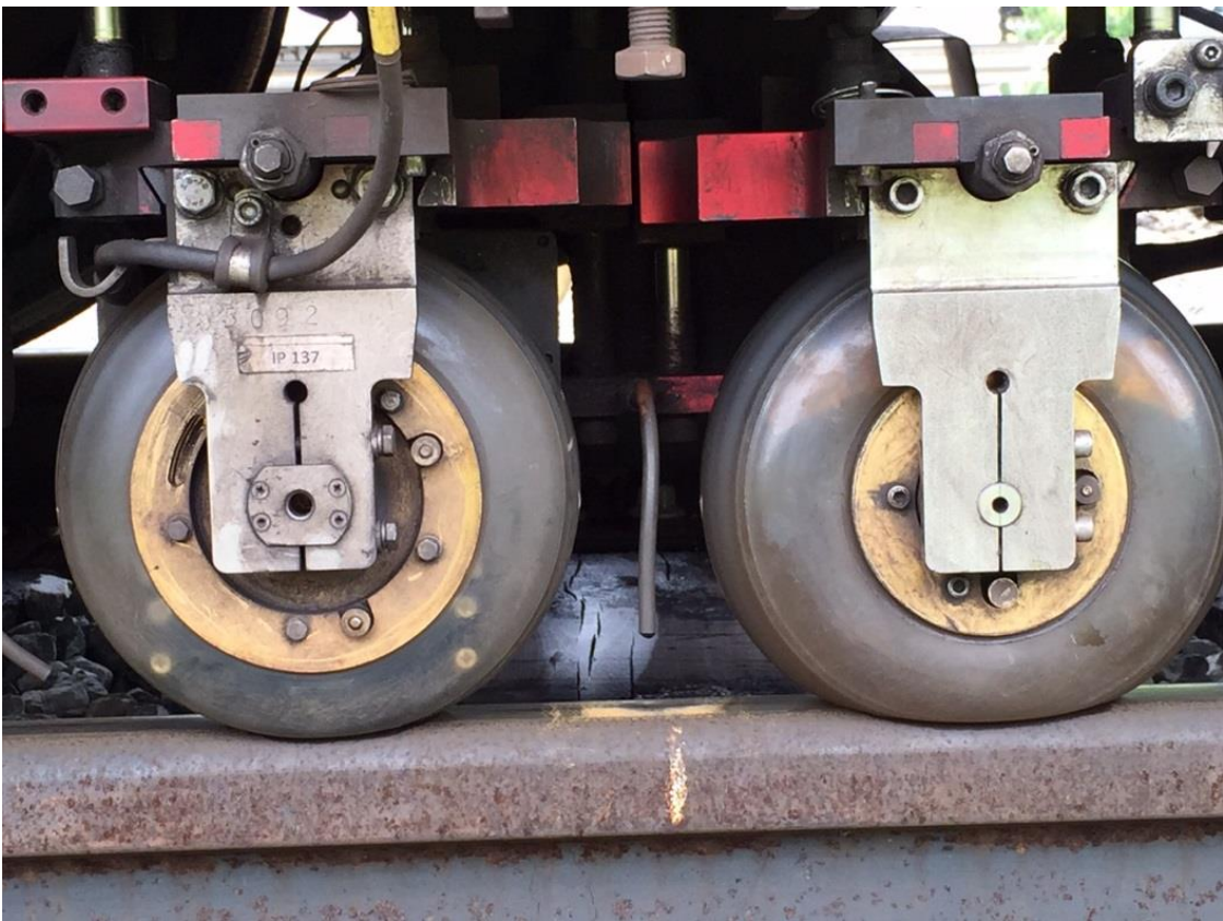
Eddy Current technology in use
