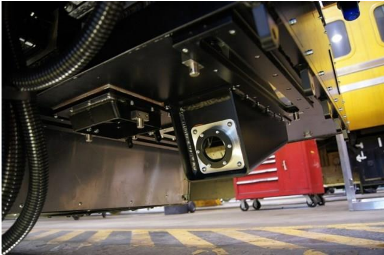
Plain Line Pattern Recognition camera
