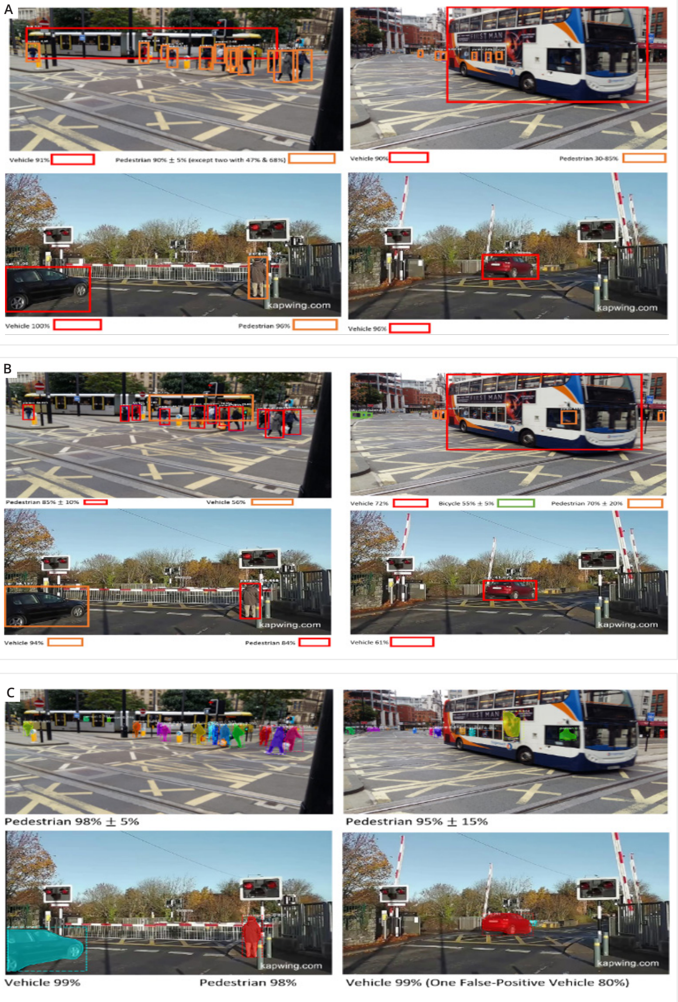
Figure 3: Predictions from: A) Yolo | B) RetinaNet | C) Mask-RCNN at two distinct environments
