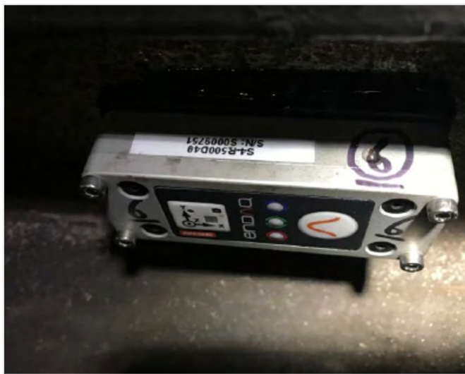
Figure 11: Stock rail fitted enDAQ Sensor
