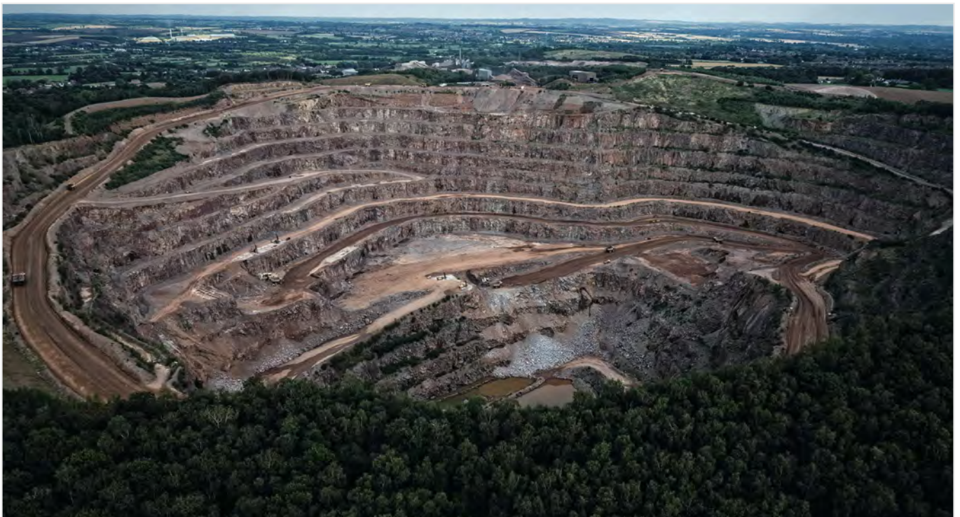
Figure 6: Tarmac's huge granite quarry at Mountsorrel. The primary crusher is visible on the far rim, beyond which are the secondary crusher, storage bins and the long conveyor to the Barrow on Soar railhead
