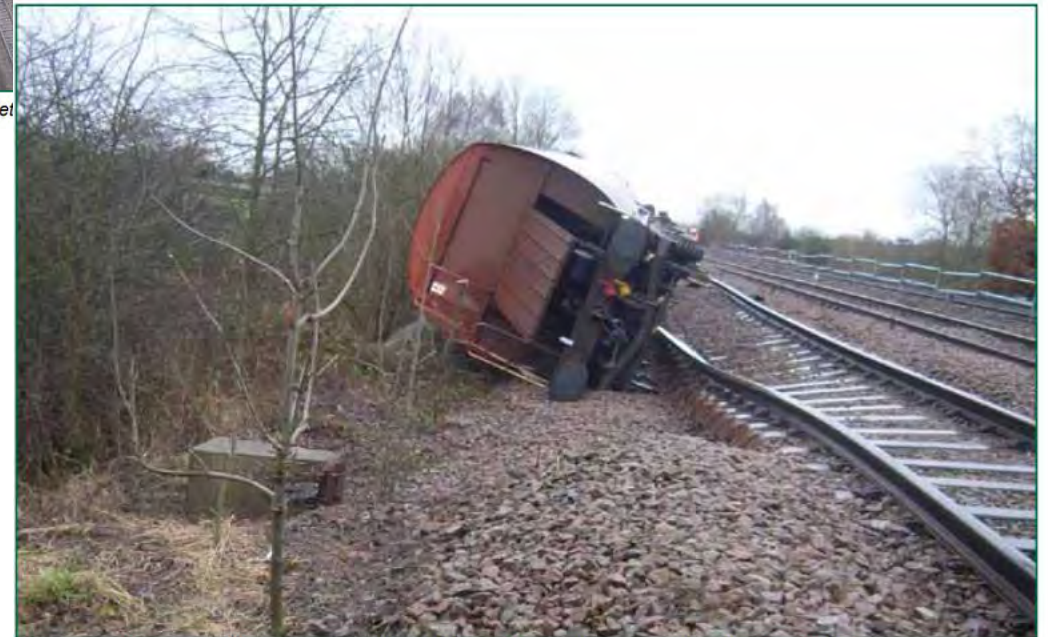
Figure 7: The rearmost wagon and loss of support under the cess rail of the Up Slow line
