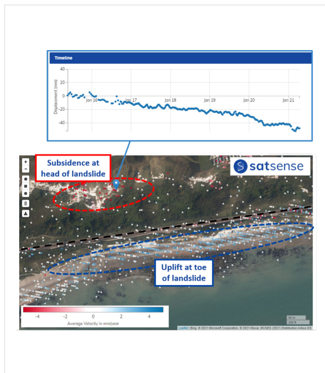
Figure 3: SatSense InSAR data showing continued landslide movement at Folkestone Warren, impacting the South East Main Line (black dashed line). The time history of a selected point shows the movement is not constant in time.
