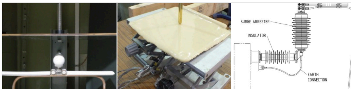
Figure 6: Insulated contact wire cover (left), polyurea coating (middle) and metal-oxide surge arrester (right).
