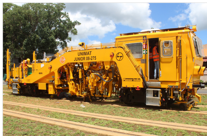
Figure 9: New Unimat Junior Tamper manufactured by Plasser, India.
