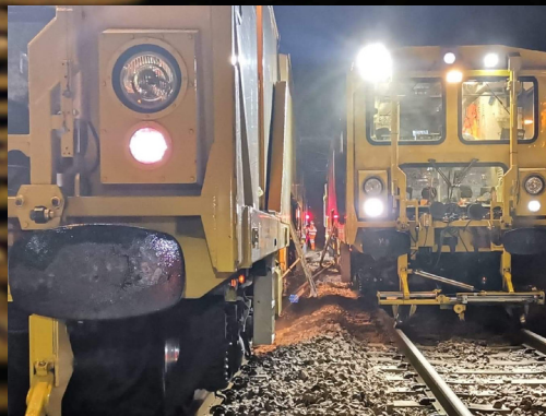
Image 3: Multipurpose stoneblowers working in tandem at Shields Jn Glasgow (Photo courtesy Neil Wightman)
