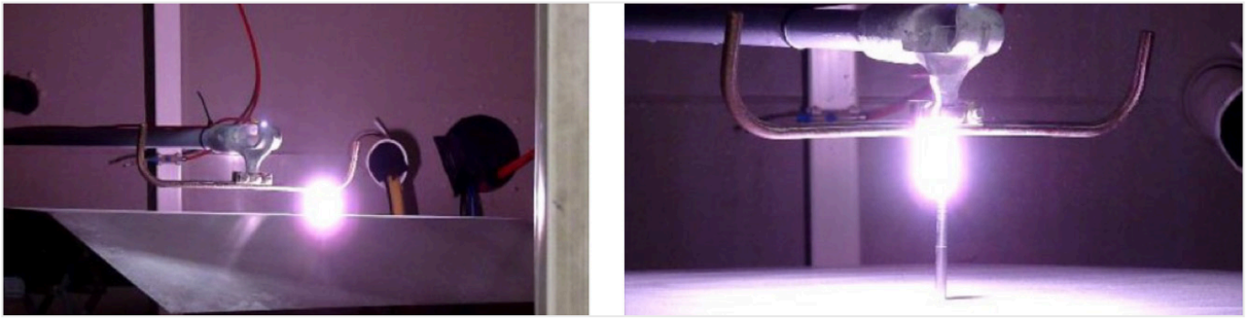
Figure 9: Flashover between contact wire and train roof (left), roof mounted aerial (right).
