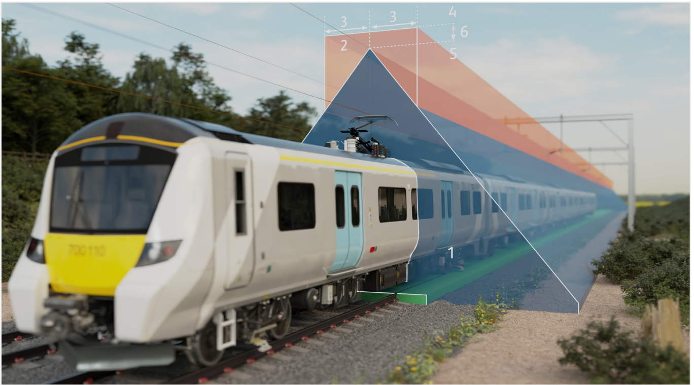
Figure 4. Overhead contact line zone (1) and current collector zone (2).
