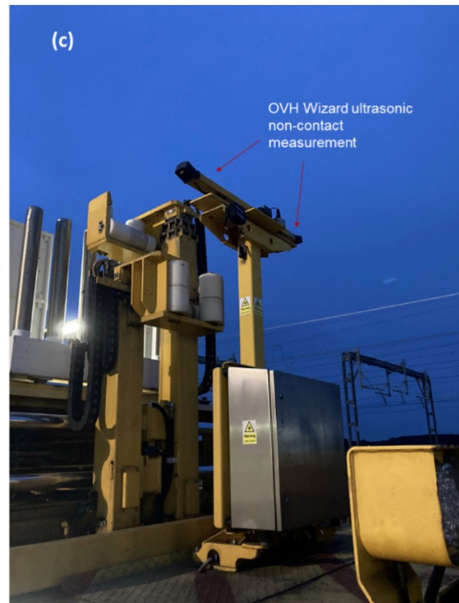
Figure 1: (a) Mentor contact interface testing NR Service train using a single BW HSA pantograph up to 100mph (tethered pantograph view from within the data acquisition cab), (b) New Measurement Train (NMT), non-contact wire profile monitoring height and stagger at \sim 250\text{mm} increments up to 1000Hz and (c) OVH wizard equipment mounted on the HOPS train monitoring height and stagger at \sim 500\text{mm} increments up to \sim 24\text{Hz} .
