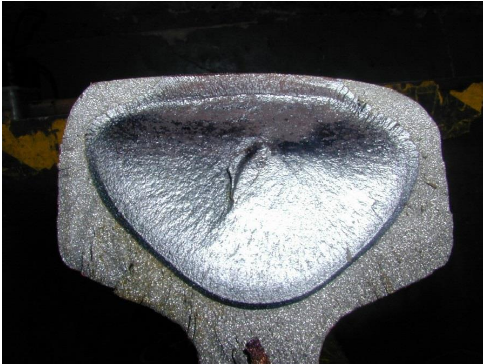
Figure 3.20 Tache Oval Failure (courtesy Jay Jaiswal)
