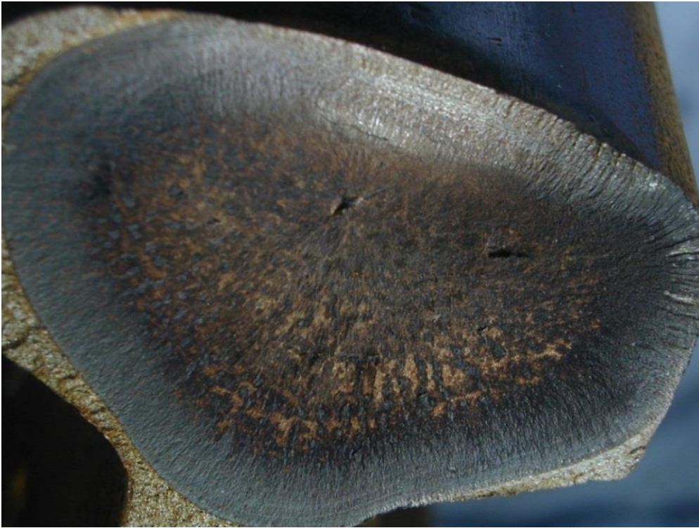
Figure 3.19 Squat failure (courtesy Jay Jaiswal)
