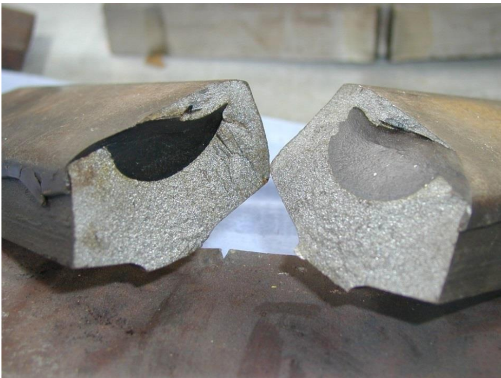
Figure 3.24 Rolling Contact Fatigue Cracking leading to Failure (courtesy Jay Jaiswal)
