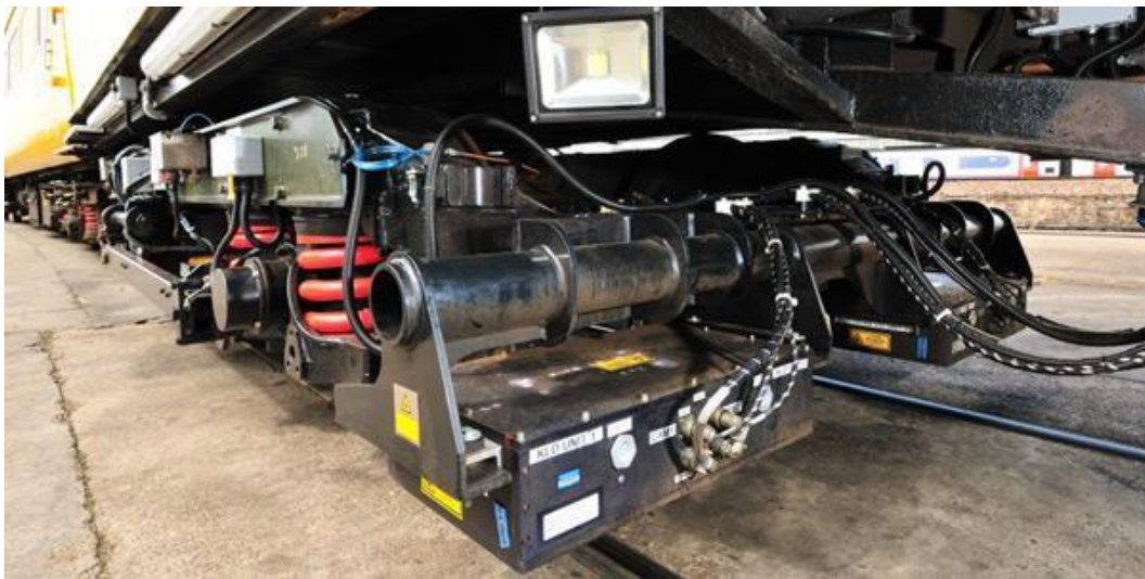
Figure 3.27 Ultrasonic equipment on UTU 2 (Courtesy of Network Rail)
