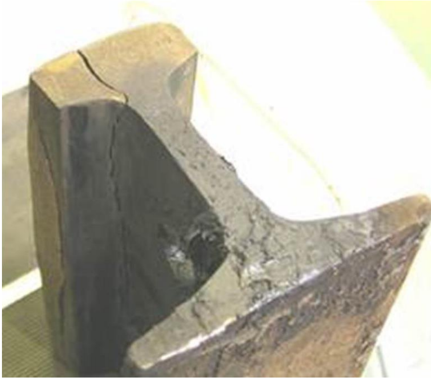
Figure 3.22 Vertical Split Failure (courtesy Jay Jaiswal)
