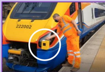
External SIG housing that fits temporarily on Tail Lamp Bracket (mounted by hand)
