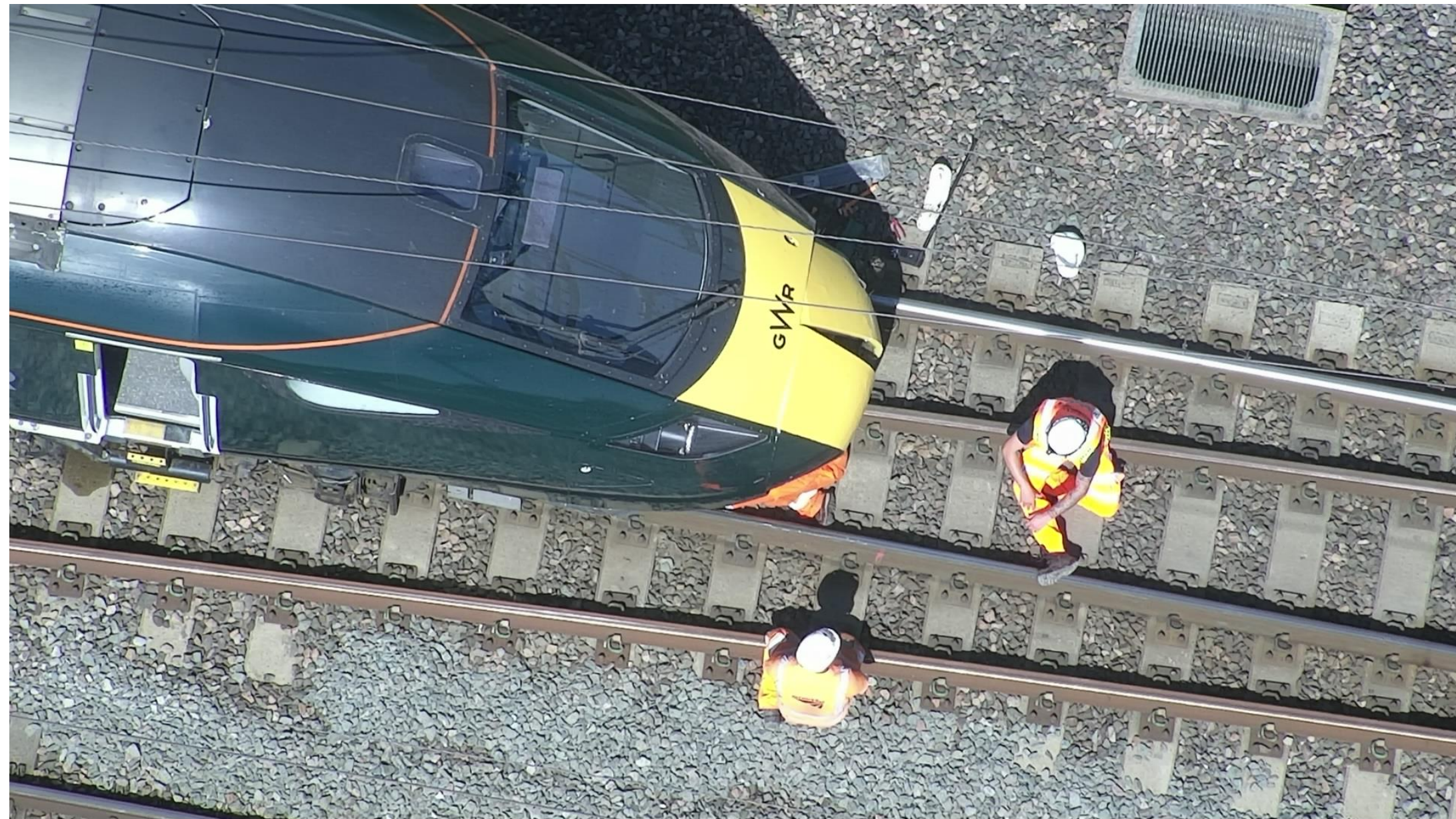
Incident Response, The Damage to this New Hitachi Train was the Result of Colliding with 7 Cows on the Main Line at Wotton Bassett
