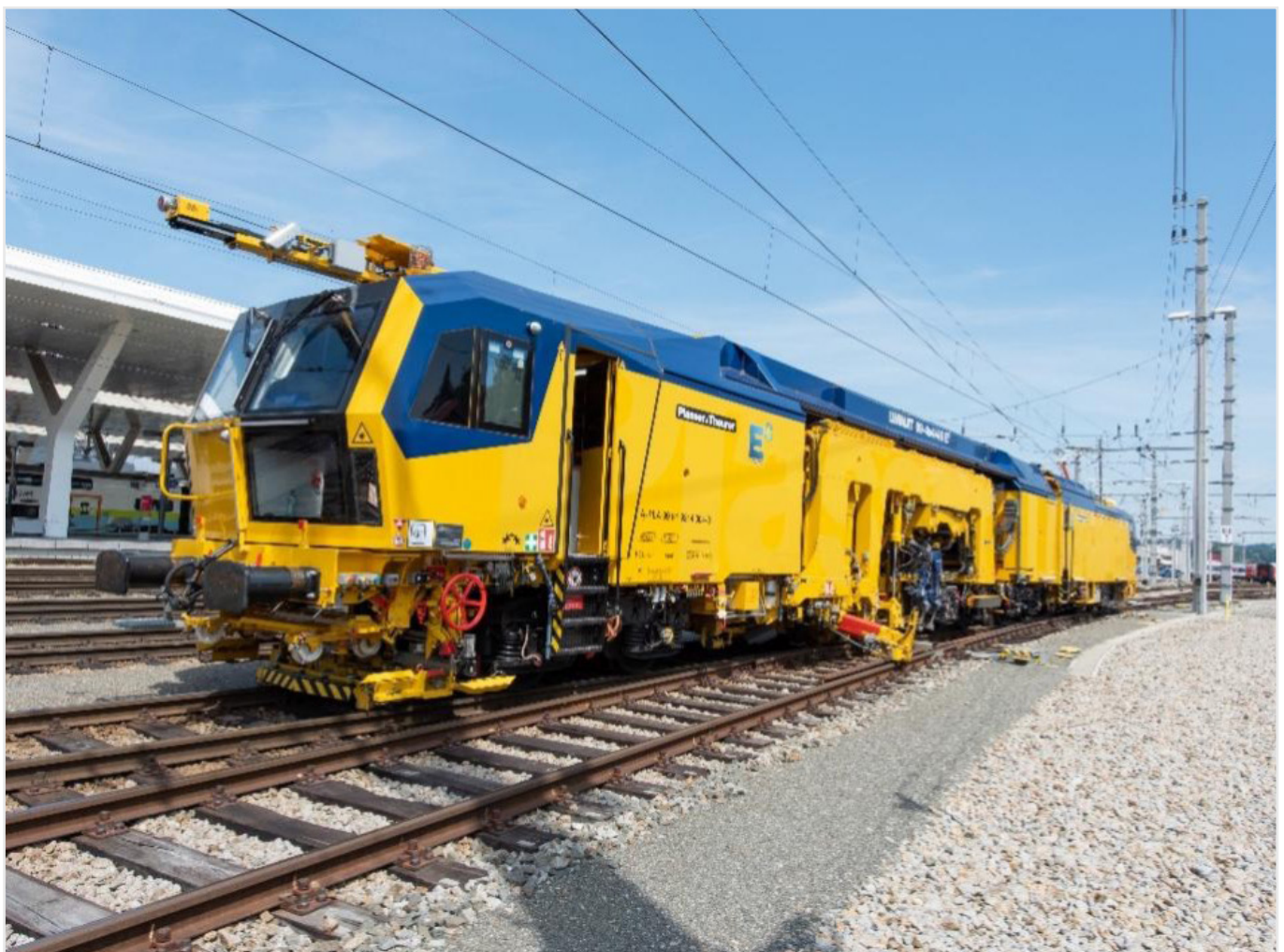
Figure 1: Tamping machine equipped with PlasserSmartTamping - The Assistant [4].
