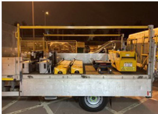
Figure 6: Two methods of transporting the Felix machine to site. Left - the modules are kept in the transport kit and the entire kit is loaded onto a truck using forklift or tail lift; right - only the individual modules are loaded.
