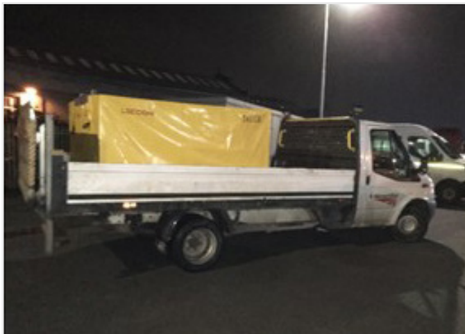
Figure 6: Two methods of transporting the Felix machine to site. Left - the modules are kept in the transport kit and the entire kit is loaded onto a truck using forklift or tail lift; right - only the individual modules are loaded.
