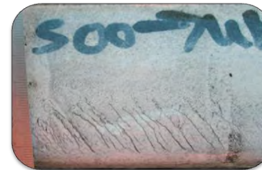
R260 - 27mm surface crack length (3 months after grinding)
