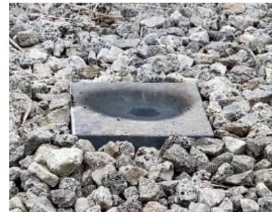
Image 4 - After removal of the flame source – sample self-extinguished
