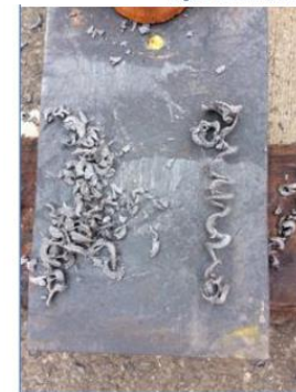
Figure 9 - Example of plastic swarf following drilling.
