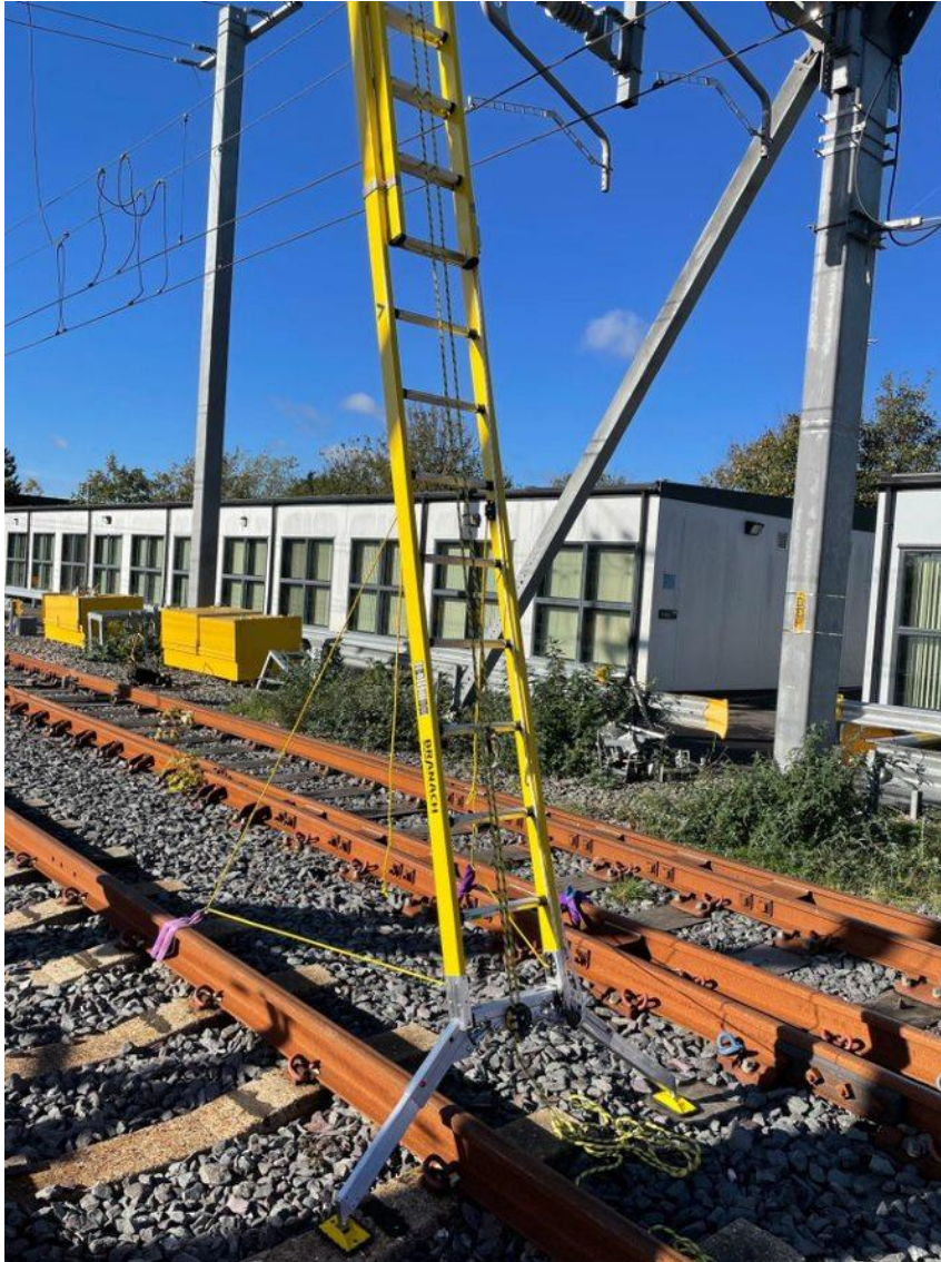
Ladder rail mounted with adjustable feet
