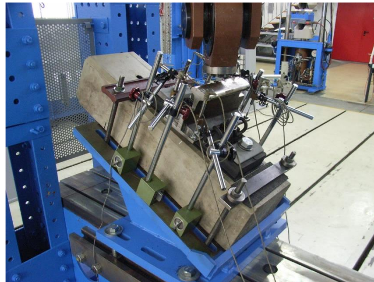
Fatigue test of fastening system acc. to EN 13481
