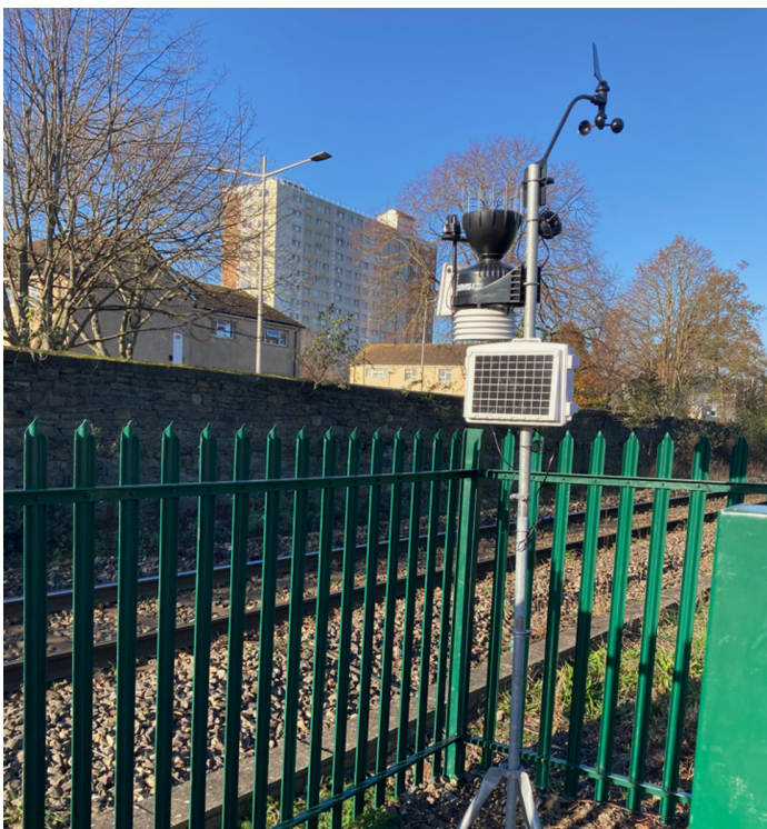
Figure 9: Davis Vantage pro 2 plus weather station in Cardiff Bay
