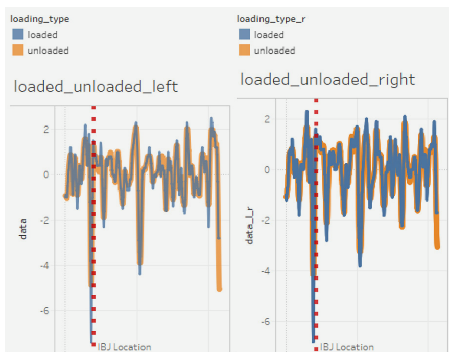
Figure 9: Loaded/Unloaded signals plotted for a section. The y-axis represents vertical deformation in mm, while the x-axis represents the position along the track.
