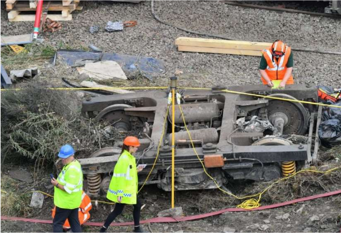
Fatal derailment at Stonehaven, Scotland in 2020. Passenger train hit a landslip following heavy rain
