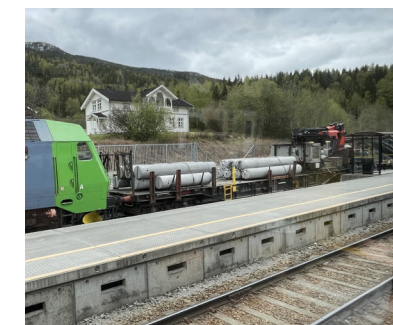
Figure 2: Concrete pile installation train.
