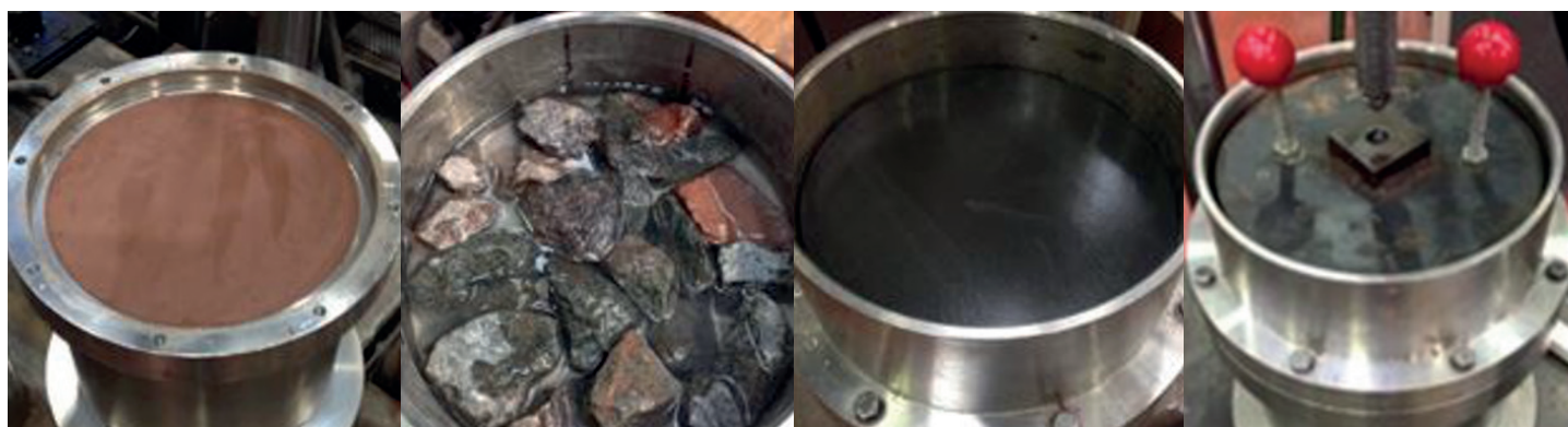
(a) Compacted subgrade. (b) Ballast inundated with water. (c) Under sleeper pad. (d) Terram cell – completed assembly.
