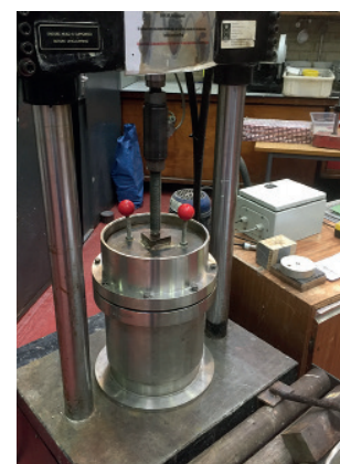
Figure 3: Set up of the Terram cell in the load frame.
