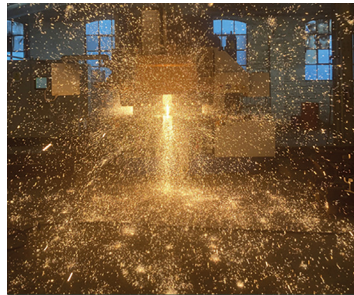
Figure 9: Flash butt welding of rail legs onto cast manganese crossing bodies in the Sheffield facility (Image courtesy of Progress Rail).
