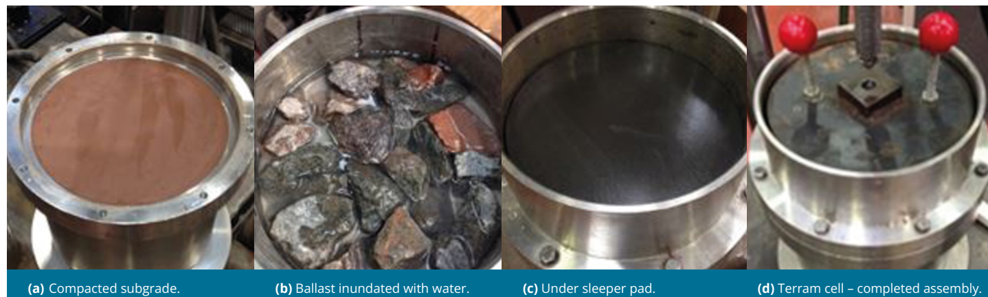
Figure 4: Key stages of the test setup.
