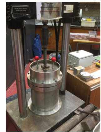
Figure 3: Set up of the Terram cell in the load frame.
