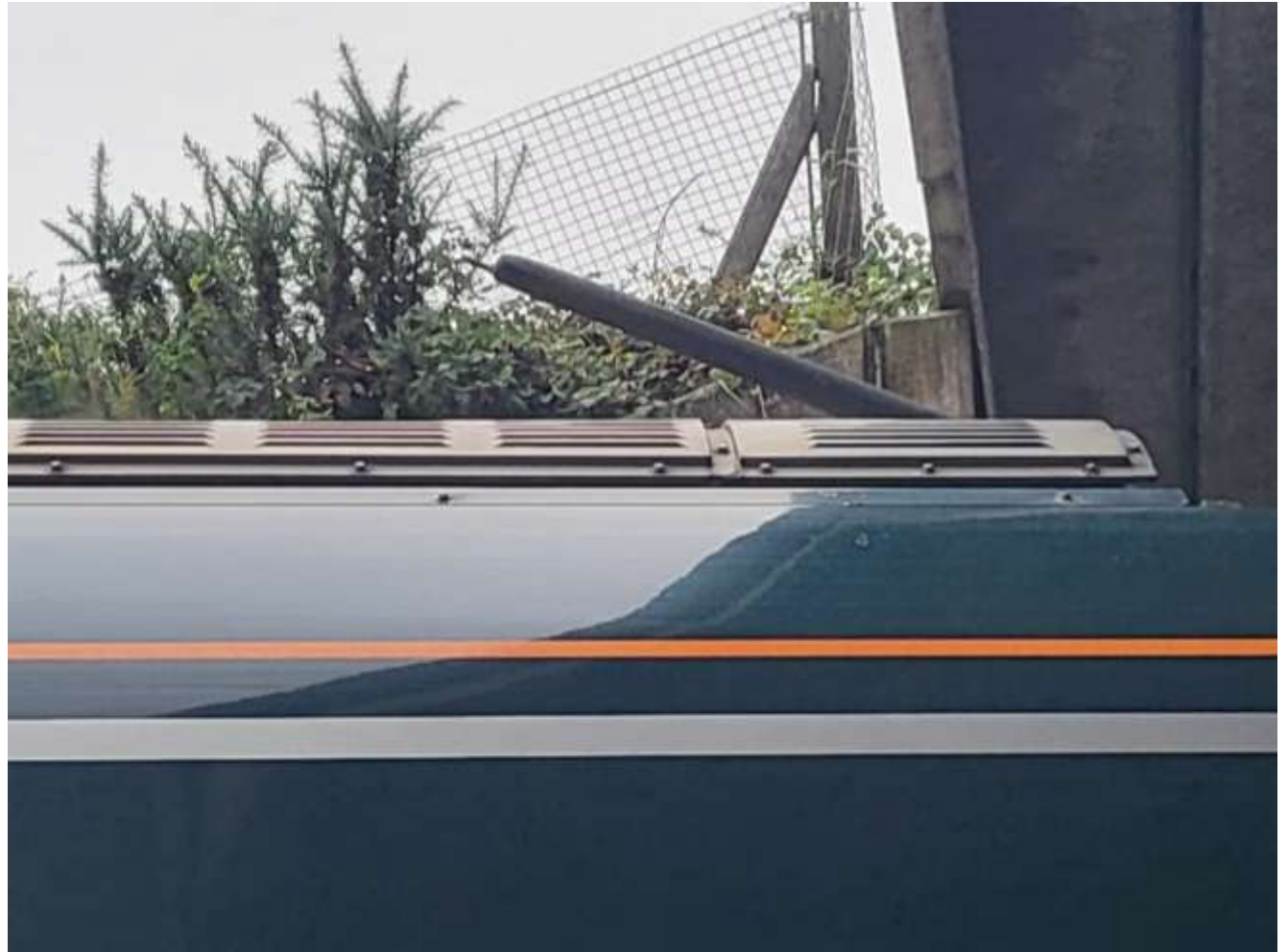
Missing pantograph upper assembly - 2024
