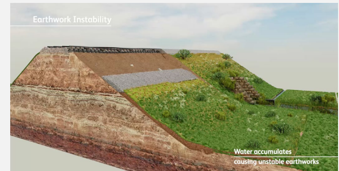
Image showing impact on earthwork from poor drainage
