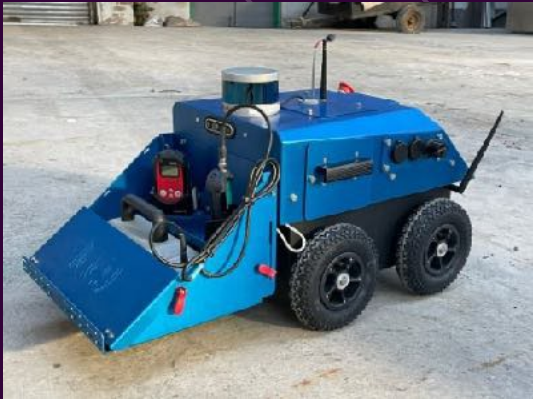
CARMA - Exploration Platform Capable of Deployment in Hazardous Confined Spaces
