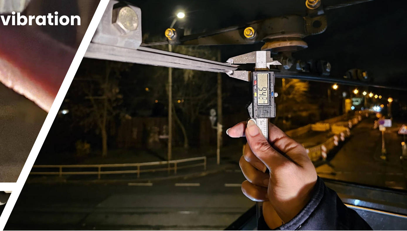
Detected low thickness
