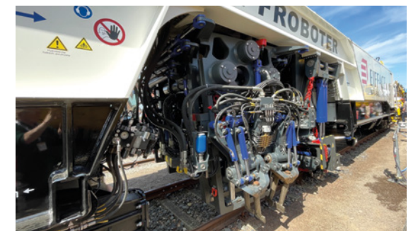
System 7 tamping banks on new machine for Eiffage.
