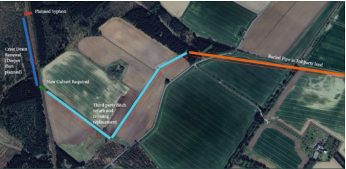
Figure 15: Alternative overland flows for syphon diversion.
