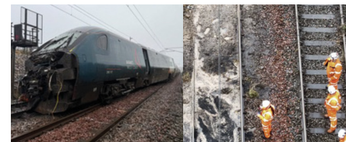
Figure 5: A landslip caused a derailment of a high speed train at Shap in Cumbria (Photo courtesy of Network Rail and RAIB).
