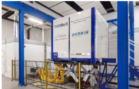
Rail vehicle high-fidelity motion simulator
