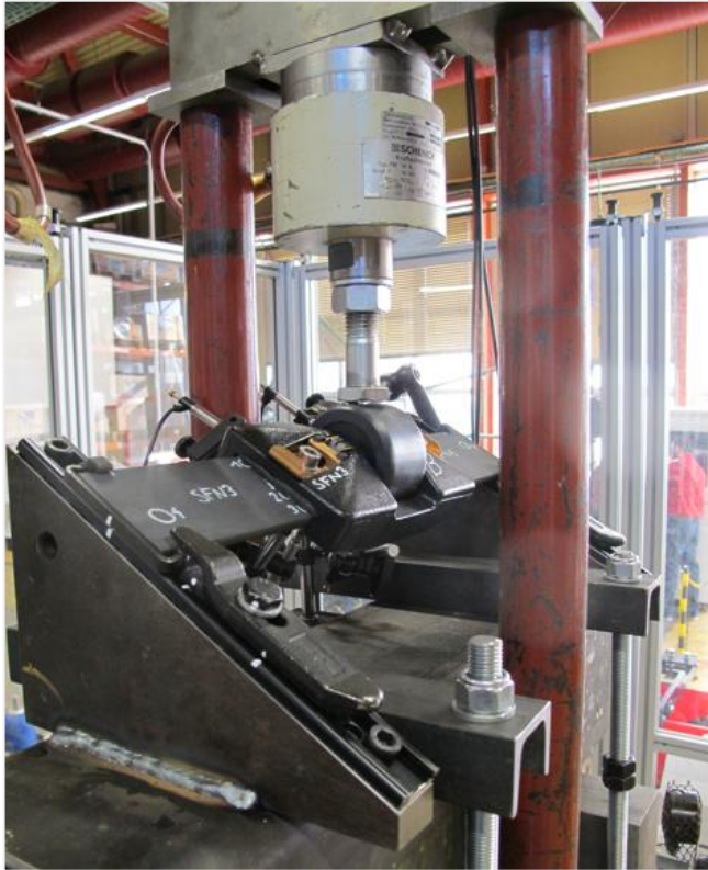
Sloping load test with inclined forces TVFA-Vienna, 10 million load cycles
