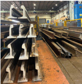
Figure 1: Main factory floor at KGJ Price, showing rolled rail machined and/or drilled ready for assembly.
