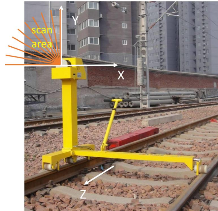
LiDAR equipment mounted on trolley
